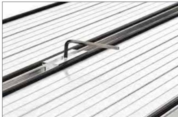
Altech Supasafe Clamps should be positioned approximately 1/3 of the plank length in from the plank ends, and can easily be fitted with an allen key
