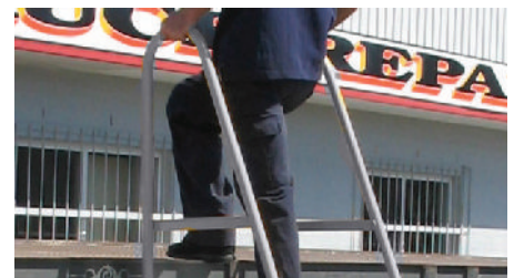
With two side safety rails to maintain a firm hand hold, access to the work place is safe and easy.
