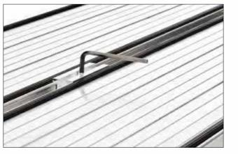
Altech Supasafe Clamps should be positioned approximately 1/3 of the plank length in from the plank ends, and can easily be fitted with an allen key
